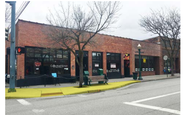
In downtown, corner curb extensions provide additional space for seating and trees (see highlighted area).
